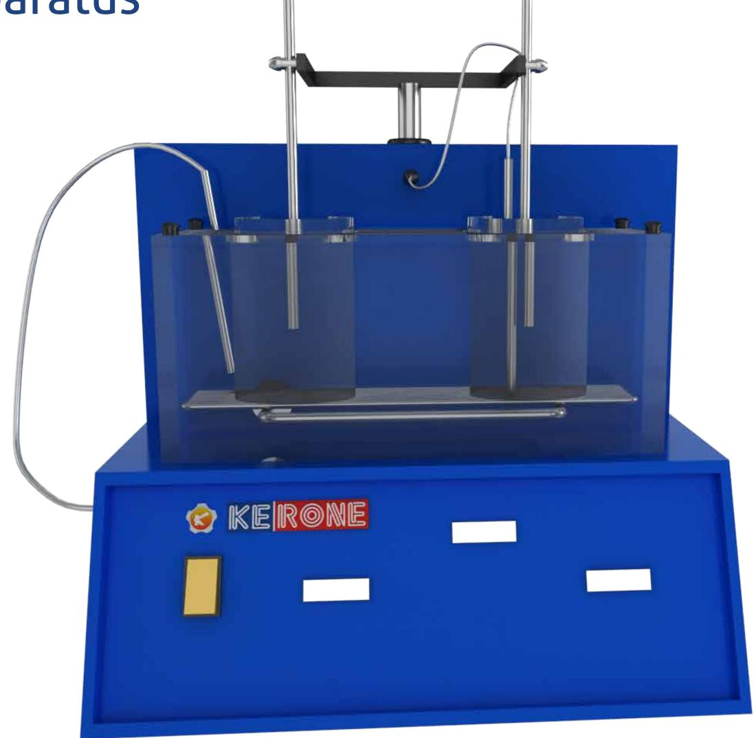
The apparatus consists of two hot plates provided to maintain the temperature of the liquid media (100 ml beaker). Solid state regular heat is provided to control the temperature of the hot plates. Two batches of six tablets each can be tested simultaneously. It provides a constant speed of 30 RPM motor drive with single bar, smooth up and down lifts for two baskets.
